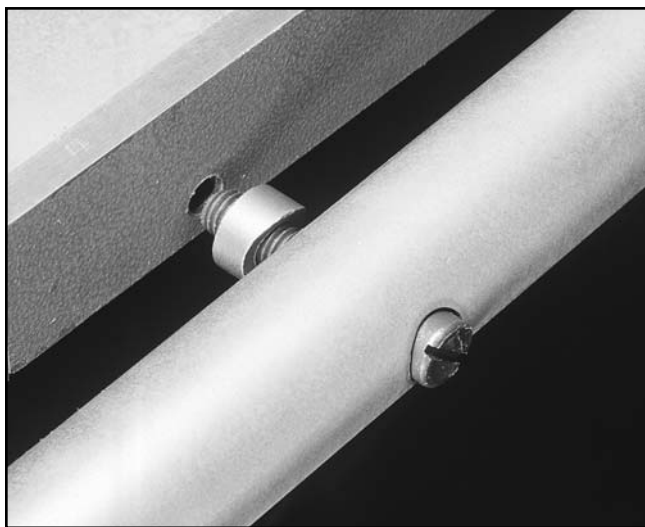
Figure 24. Attaching fence rails.
